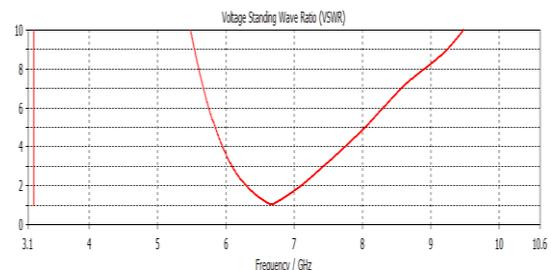
**Fig. 5.** VSWR versus frequency plot for the proposed half wave dipole antenna.
