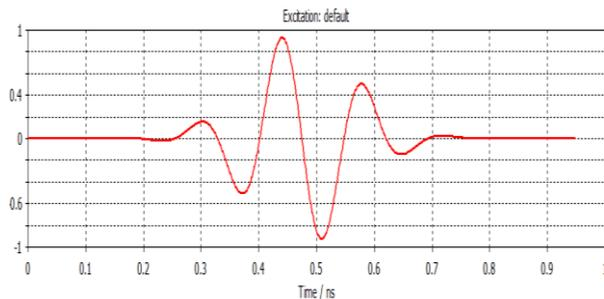
**Fig. 2.** Excitation Signal-Gaussian Pulse.
