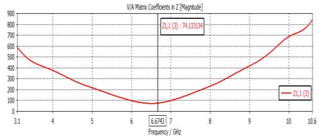
**Fig. 3.** Impedance characteristic of the proposed half wave dipole antenna.
