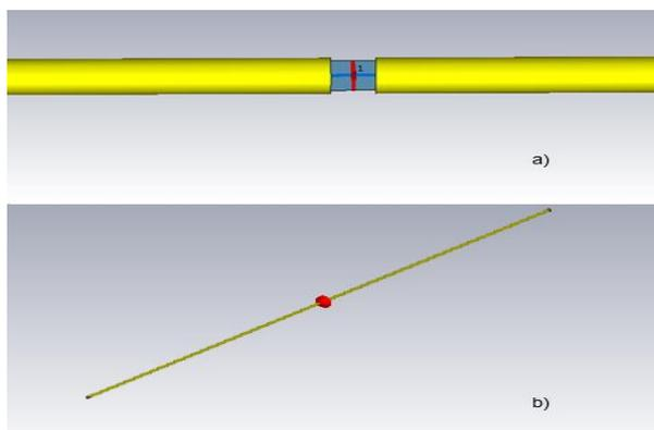
**Fig. 1.** Half Wave Dipole Antenna Geometry
