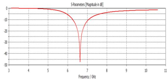
**Fig. 4.** Return loss characteristic of the half wave dipole antenna.
