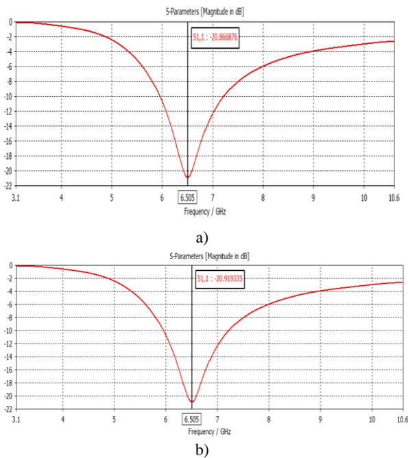
**Fig. 8.** Return Loss Characteristics of the half wave dipole antenna by using a) PSO b) GA with 25 iterations.
