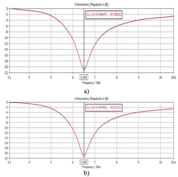
**Fig. 10.** Return Loss Characteristics of the half wave dipole antenna by using a) PSO b) GA with 261 iterations.
