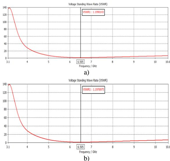
**Fig. 9.** VSWR Characteristics of the half wave dipole antenna by using a) PSO b) GA with 25 iterations.
