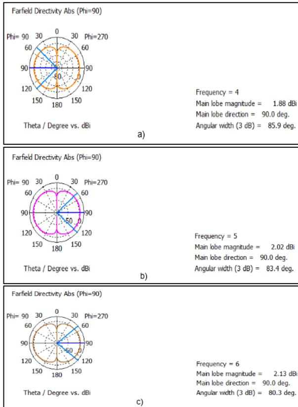
**Fig. 6.** Radiation Pattern for half wave dipole antenna with frequency a) 4 GHz b) 5 GHz c) 6 GHz, respectively.
