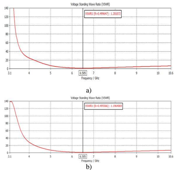
**Fig. 11.** VSWR Characteristics of the half wave dipole antenna by using a) PSO b) GA with 261 iterations.
